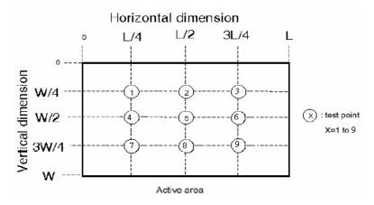
$$\left(\begin{array}{c} \text{1-} & \frac{\text{MAX Luminance} - \text{Average Luminance}}{\text{Average Luminance}} \\ \end{array}\right) \quad \text{x100\%} \quad \geq 70\%$$
