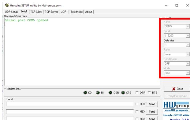
You must send a specific frame in order to move the device to configuration mode. Frame expressed in hexadecimals: 0x2B 0x2B 0x2B or « +++ ».
