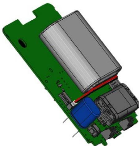
3. To close the enclosure, insert the bottom of the front panel first and snap the top of the enclosure
