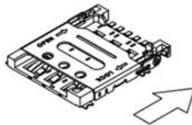
5. Open the metal cover to allow for the insertion of the Nano SIM card
