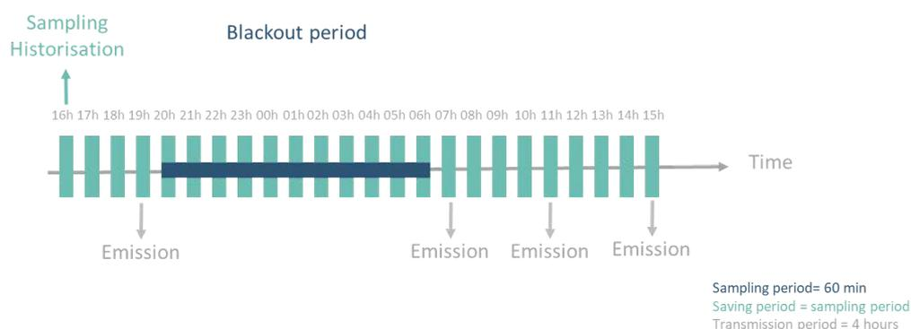
With the blackout mechanism, the product sends its last message to the server at 19:05 (7:05 PM) with the measured values at 16:00 (4:00 PM), 17:00 (5:00 PM), 18:00 (6:00 PM), and 19:00 (7:00 PM). At 20:00 (8:00 PM), the product enters the blackout period. It does not communicate until the end of the period and resumes communication at 07:05 (7:05 AM).
