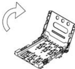
6. Place the Nano SIM card against the contacts, with the chip facing down
