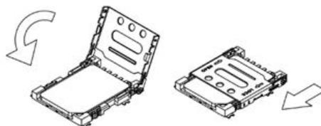
8. Place the electronic card back into the front face of the casing
