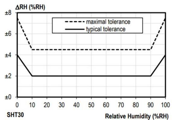
Figure 2 : Relative humidity tolerance at 25°C
