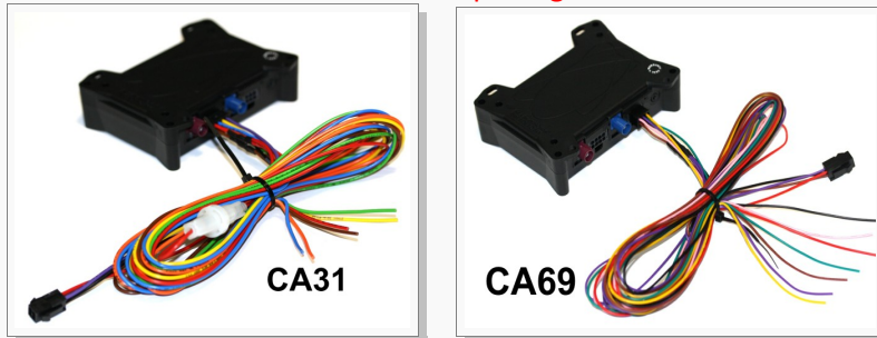
Figure 13: Supplied cables (a reference to the colours and pinout is provided in Table 7 and Table 8 )
