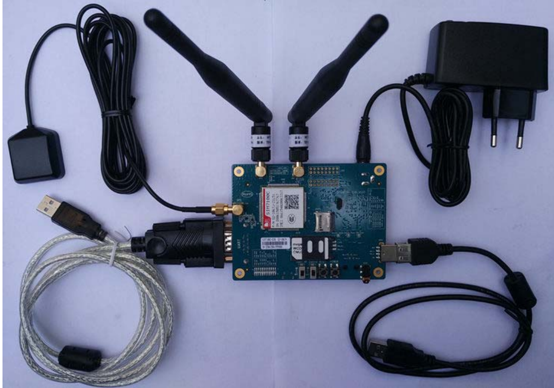
Figure 4: The assembly diagram of the EVB and Accessories
