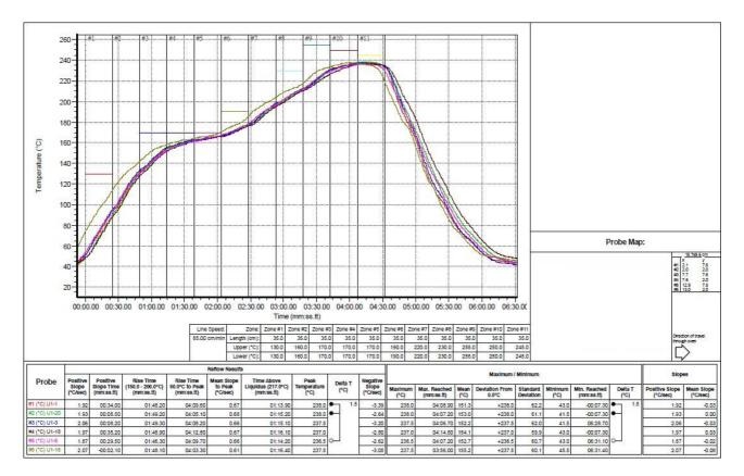
Note: Allowable reflow soldering times: 2 times base on recommended reflow profile.
