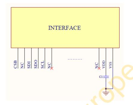
Pin connected to MCU interface: CSB, SDI,SDO, SCL
