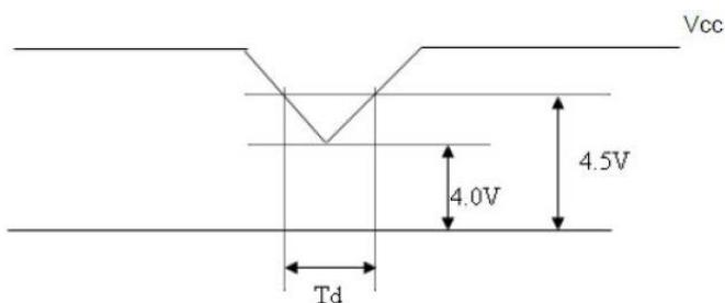
Dip condition:  $4.0 \leq V_{cc} \leq 4.5$ ,  $T_d \leq 20ms$
