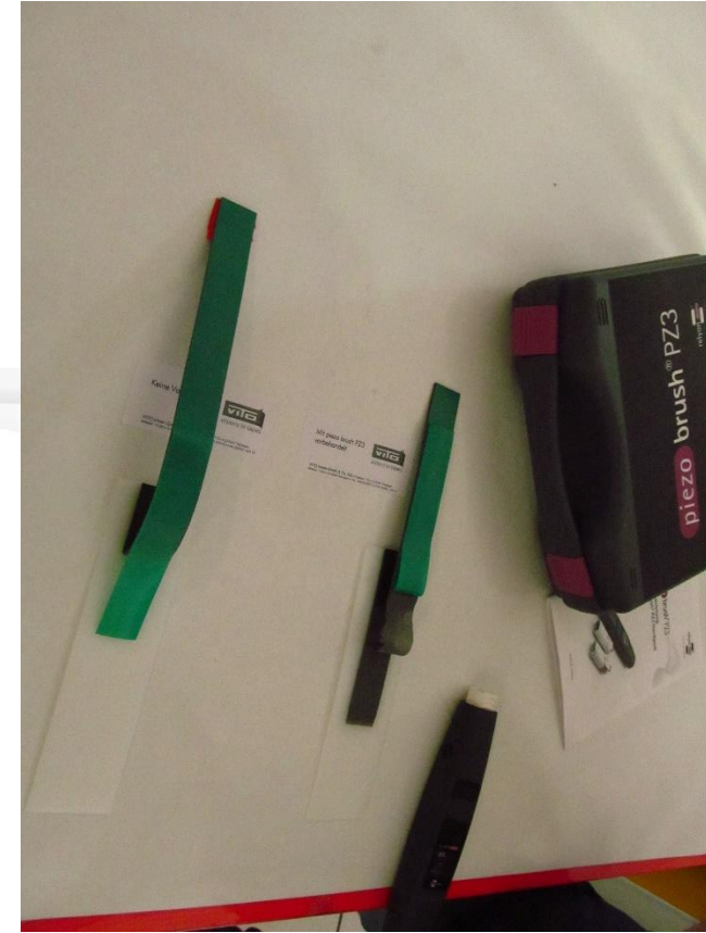
Cohesive failure of plasma treated sample
