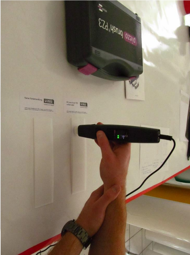
Surface treatment with piezobrush® PZ3
