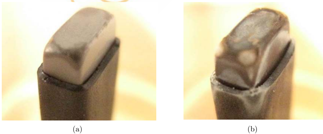
Figure 11: The tip of the CeraPlas ® F from the standard module a) before and b) after 6000 operation hours.
