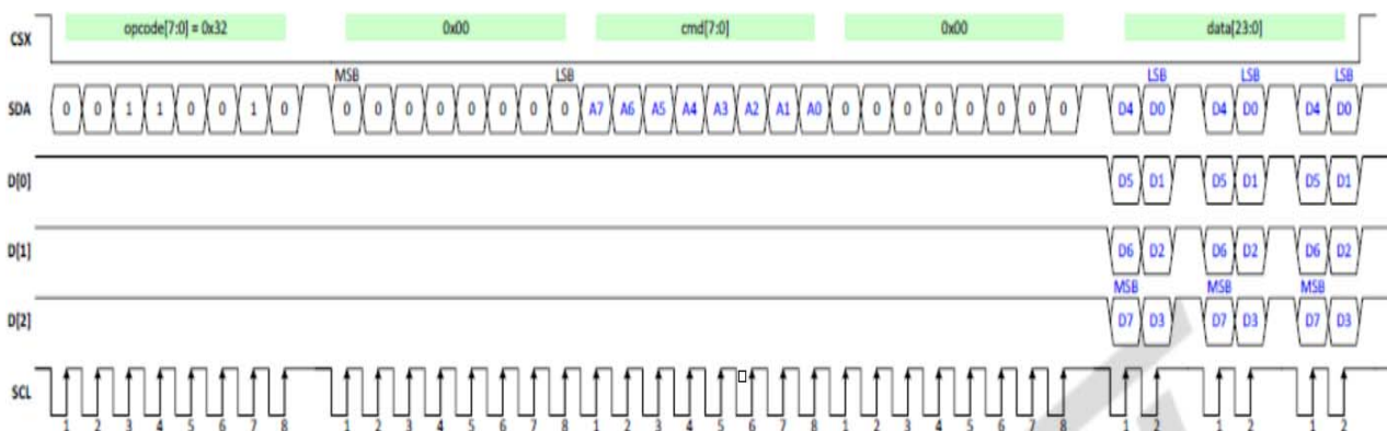
QSPI write command and write data (4 data lanes)
