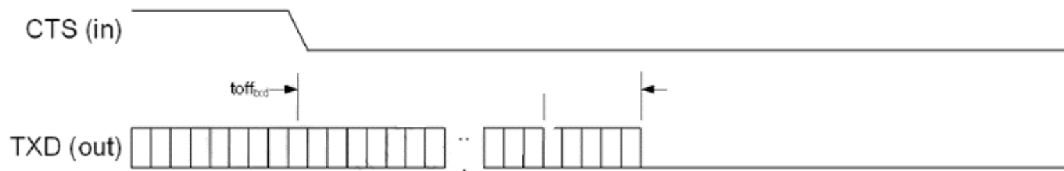
Figure 8-1: HCI UART transmit flow control timing
