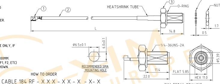
"L" LENGTH IN MM: eq: 100MM = 100 (MIN. 050-MAX.400 STANDARD = 100.150.200Tolerance: 50-200mm: ±5mm.
