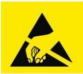
The product may be damaged by ESD, which can cause performance degradation or device failure! We recommend handling the device only on a static safe work station. Precaution for the storage should also be taken.
