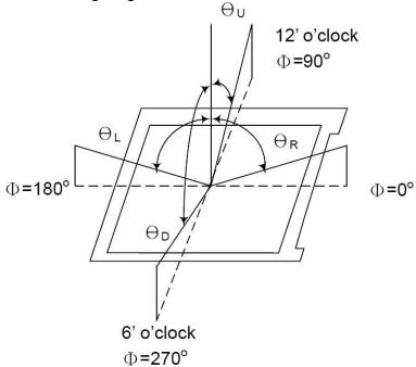
Note (2) Definition of Contrast Ratio(CR) :Measured at the center point of panel CR = Luminance with all pixels white / Luminance with all pixels black Note (3) Definition of Response Time : Sum of TR and TF
