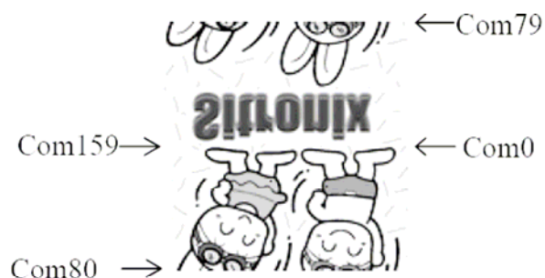
Figure 8.1.1 Common scan direction configuration
