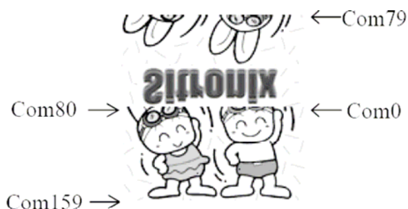
Figure 8.1.1 Common scan direction configuration
